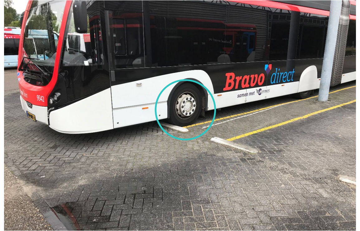
A bumper on the pavement stops the bus for the proper alignment with the hood.
